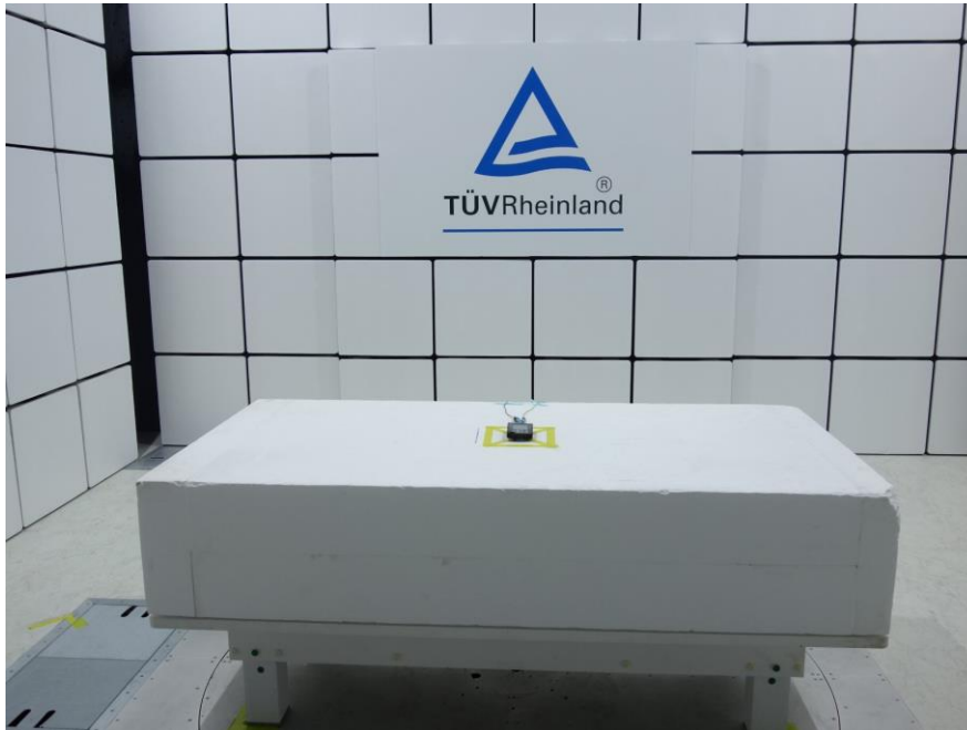
Photograph 1: Set-up for Spurious Emissions (Front View 1)
