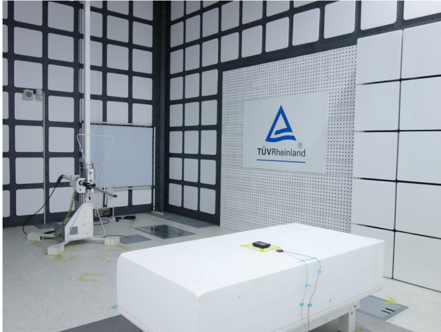
Photograph 5: Set-up for Spurious Emissions (Back View 3)
