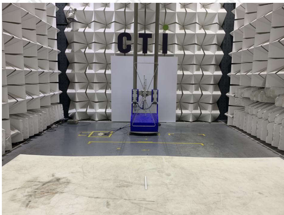
Radiated spurious emission Test Setup-1(Below 1GHz)
