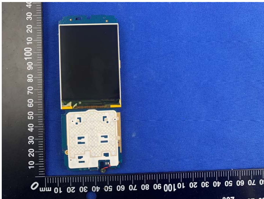
MAIN BOARD REAR VIEW (WITH SHIELDING)
