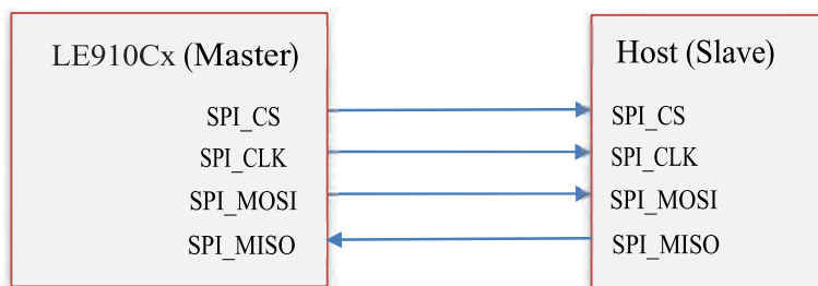
Figure 19: SPI Signal Connectivity
