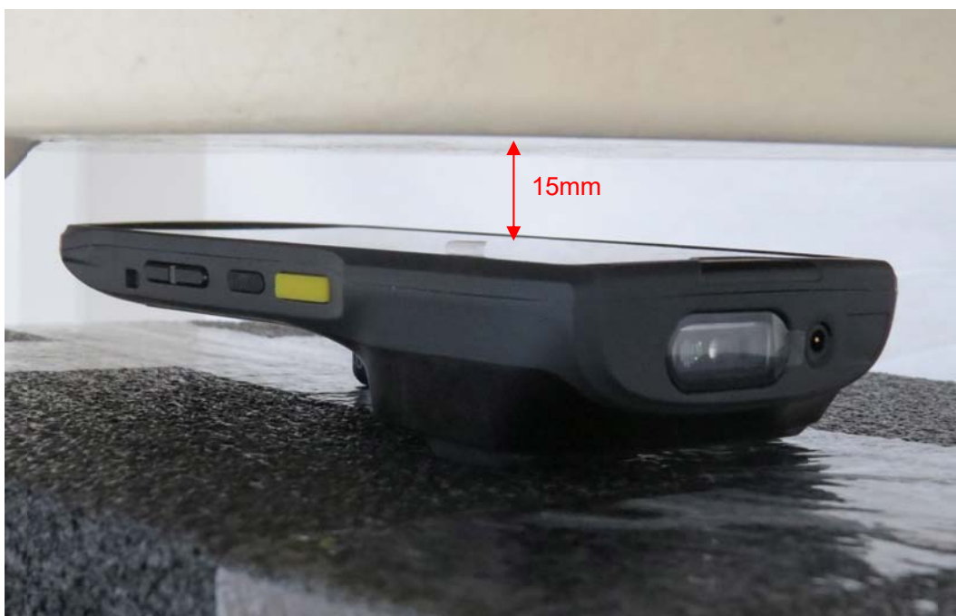
Picture 2: Front Side, the distance from handset to the bottom of the Phantom is 15mm
