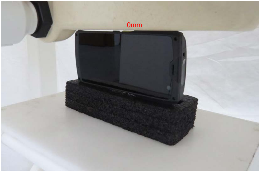
Picture 5: Left Side, the distance from handset to the bottom of the Phantom is 0mm
