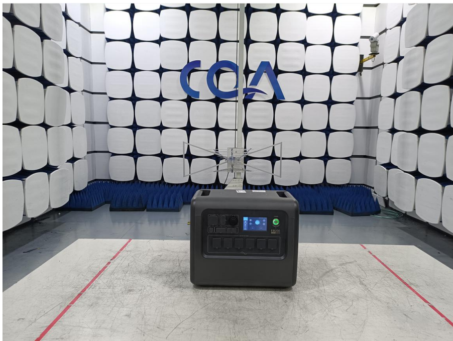
Radiated Emission below 1GHz
