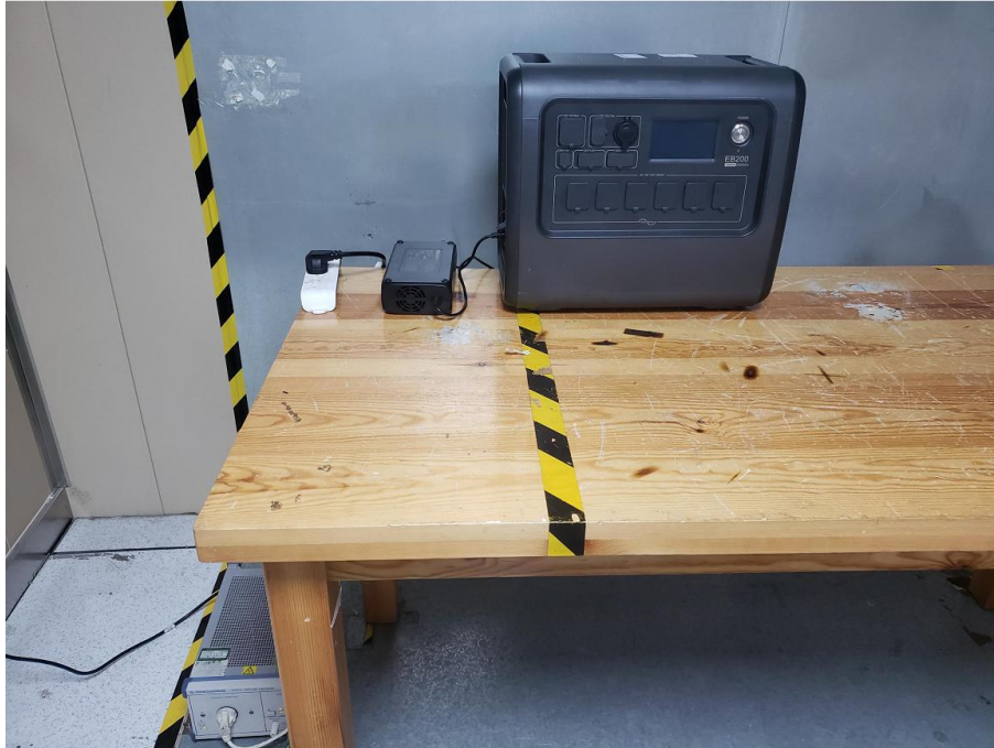
Radiated Emission below 1GHz
