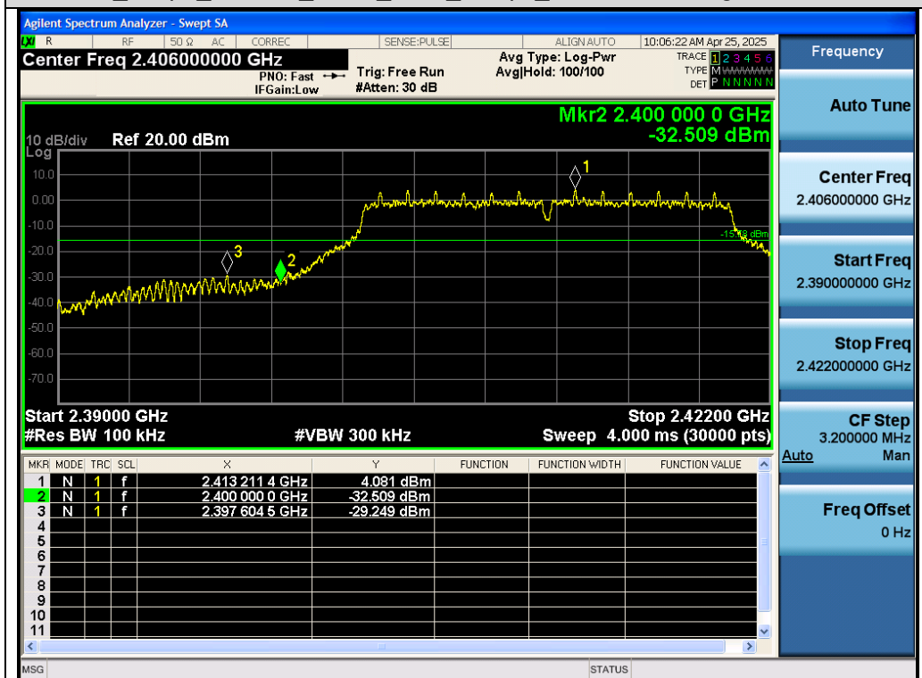
Test_Graph_802.11g_ANT1_2412_6Mbps_Lower Band Edge Emissions
