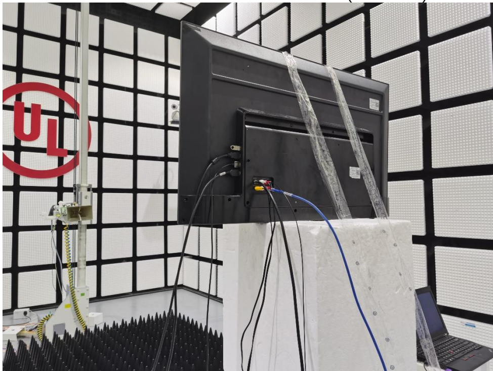
RADIATED RF MEASUREMENT SETUP (Above 1G )
