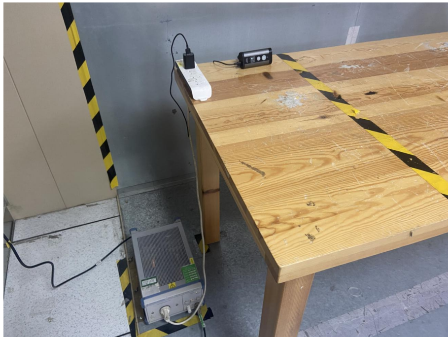
Conducted emission Test Setup
