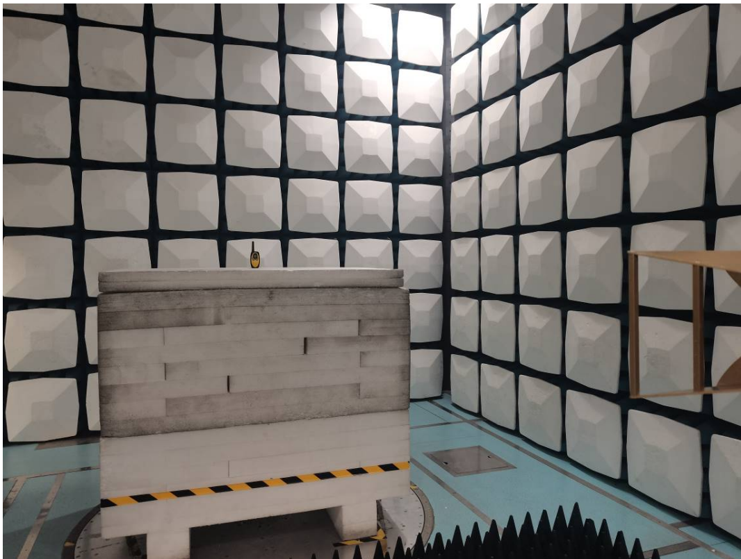
Radiated Emission Above 1GHz View
