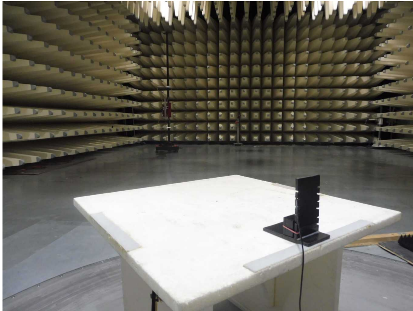
Photo 1: EUT at the semi-anechoic chamber
