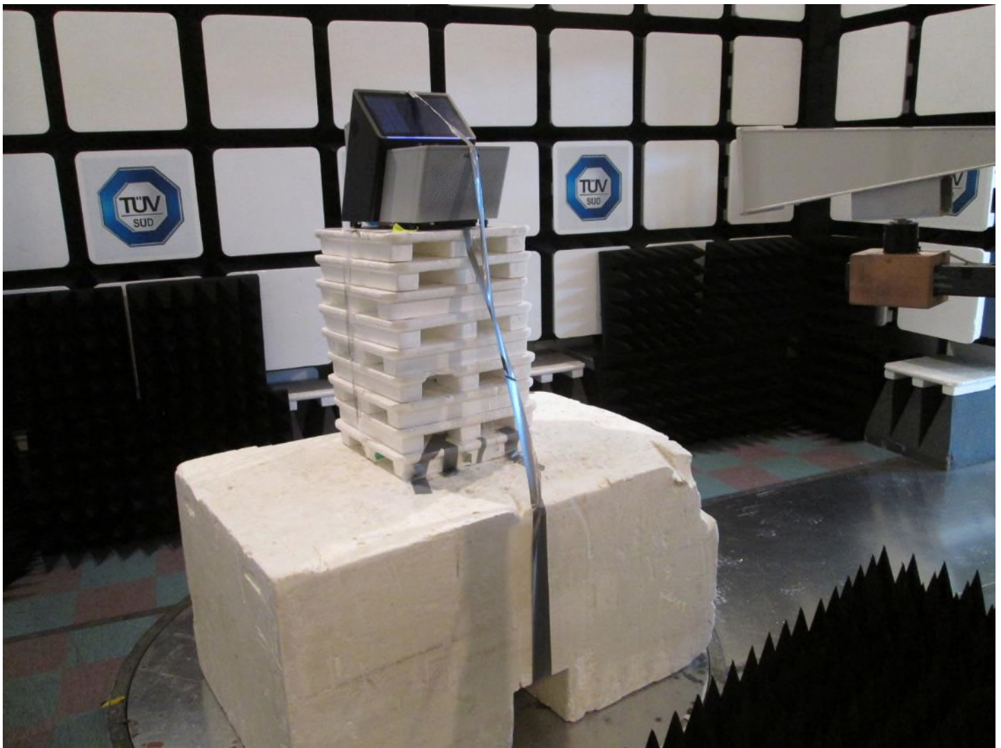
Test setup photo 5 Radiated measurements, 10 GHz – 18 GHz
