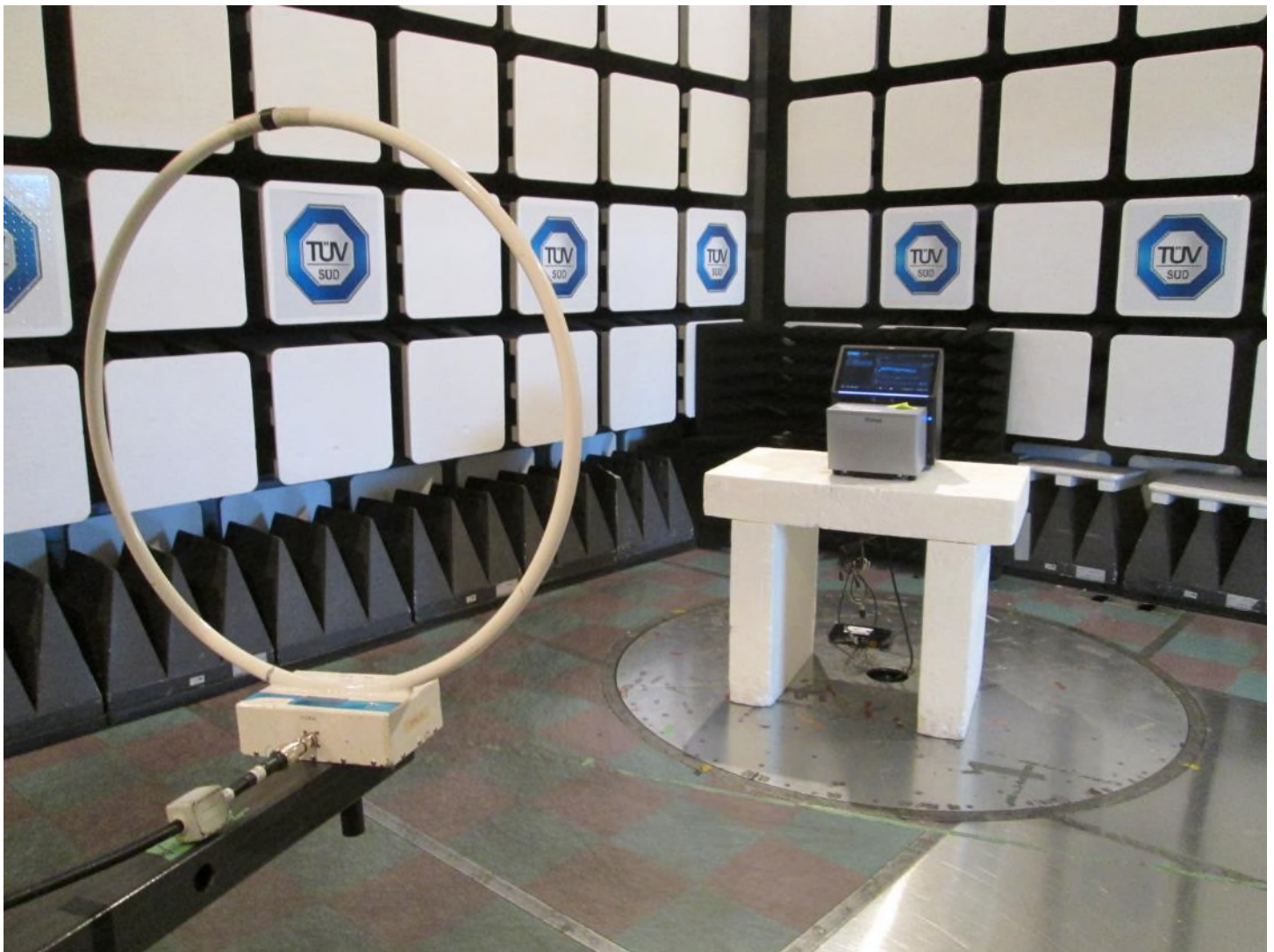
Test setup photo 1 Radiated measurements, 9 kHz – 30 MHz
