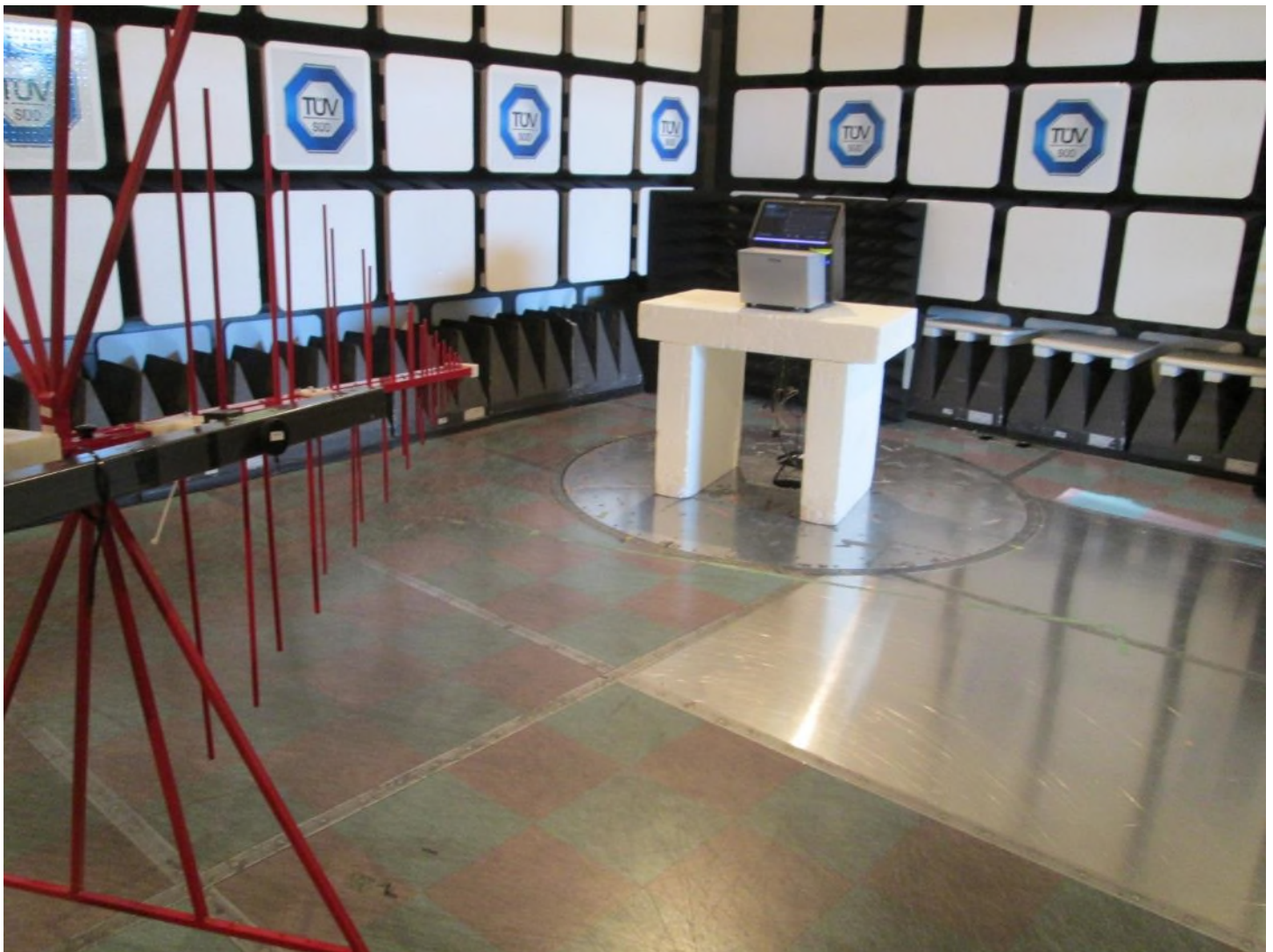
Test setup photo 2 Radiated measurements, 30 MHz – 1 GHz
