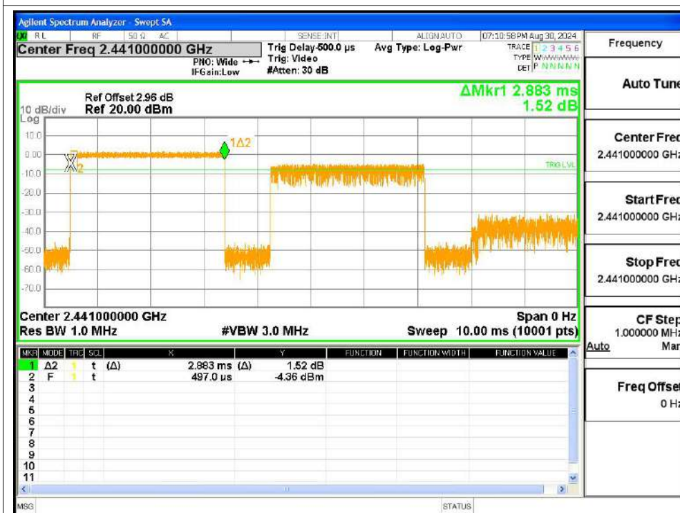
Dwell NVNT 3-DH5 2441MHz Ant1 Accumulated
