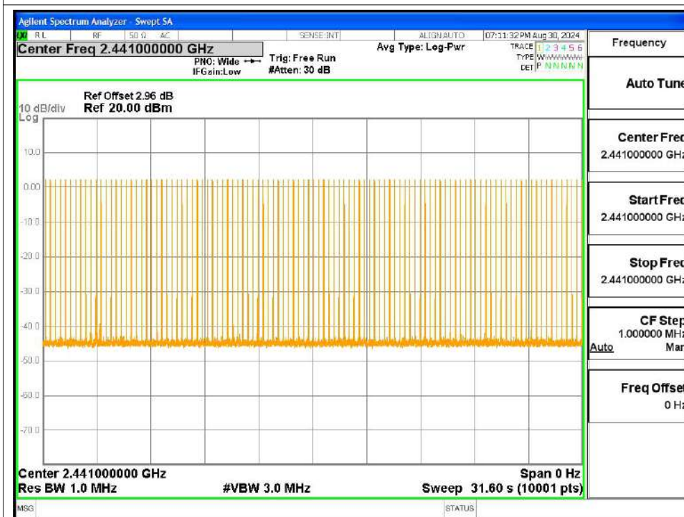
Dwell NVNT 3-DH5 2441MHz Ant1 Accumulated
