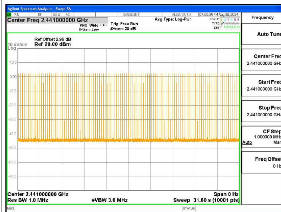
Dwell NVNT 2-DH5 2441MHz Ant1 Accumulated
