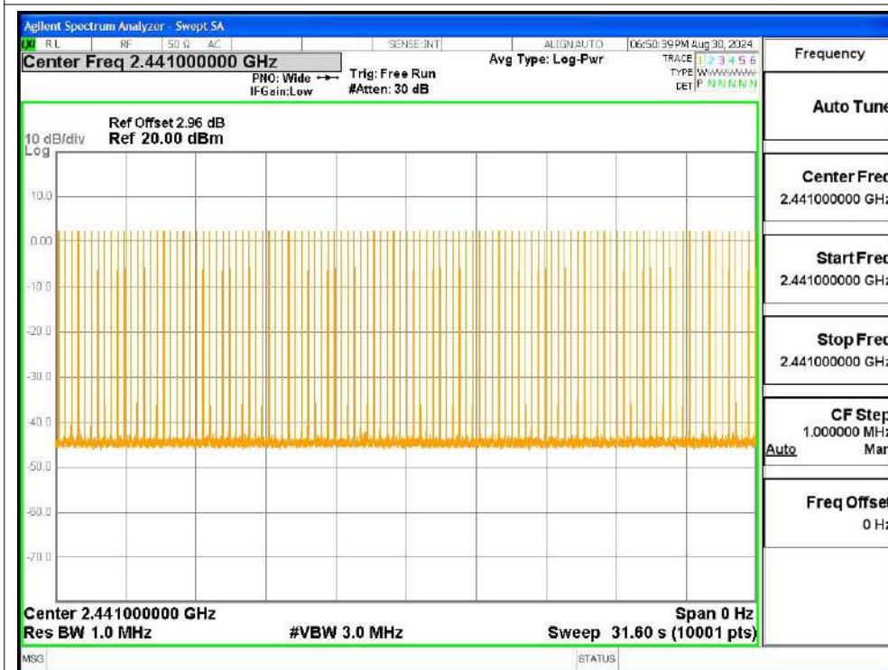
Dwell NVNT 1-DH5 2441MHz Ant1 Accumulated
