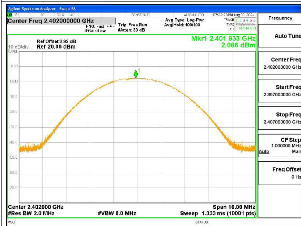
Power NVNT 2-DH5 2402MHz Ant1
