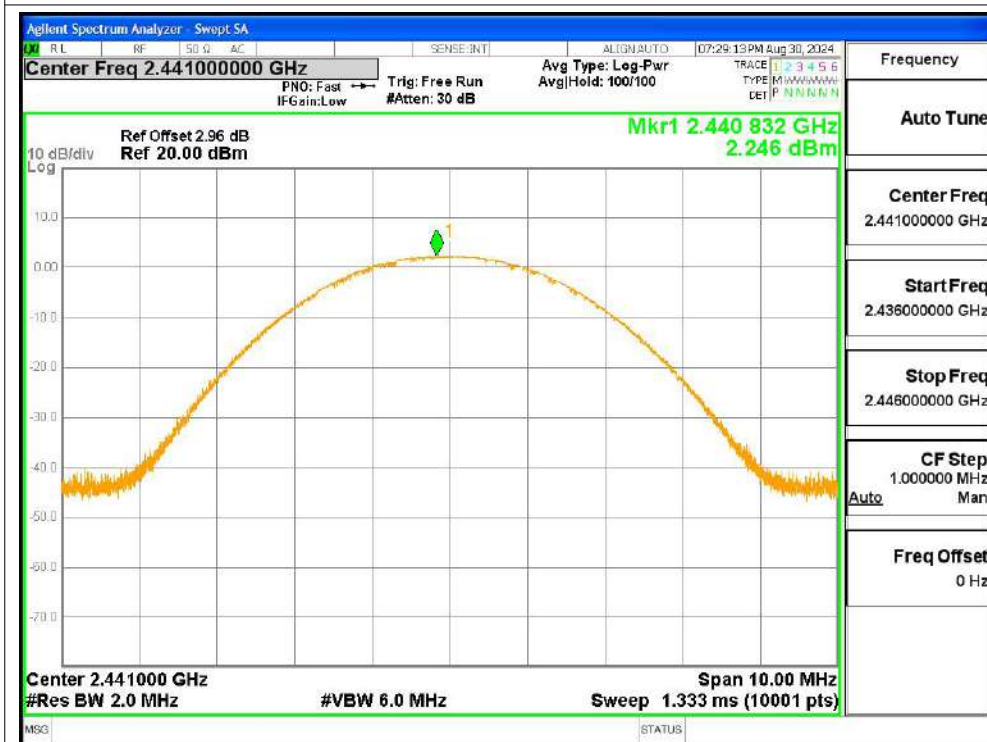
Power NVNT 3-DH5 2441MHz Ant1
