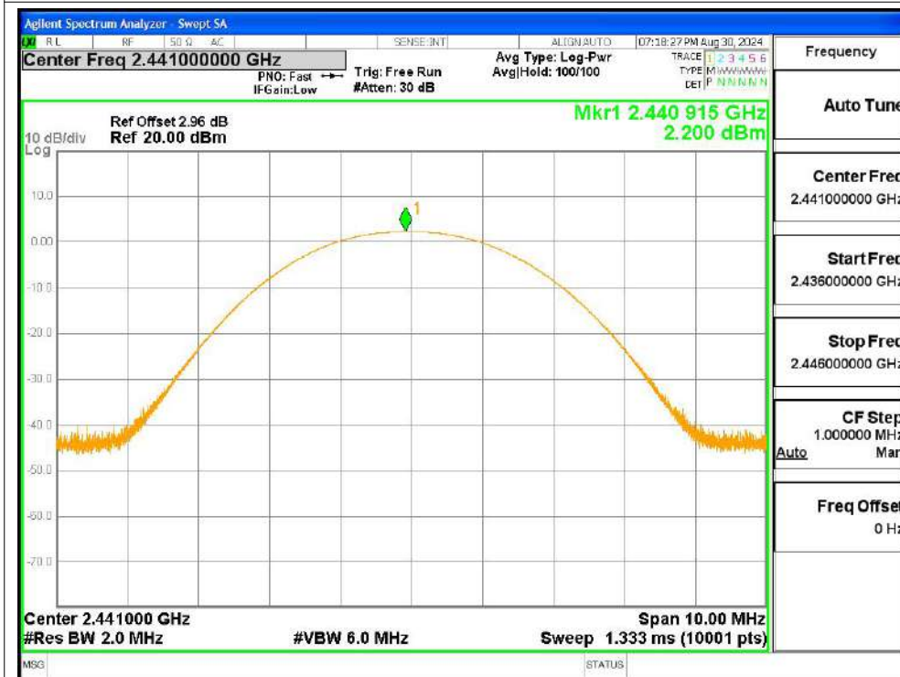
Power NVNT 1-DH5 2441MHz Ant1
