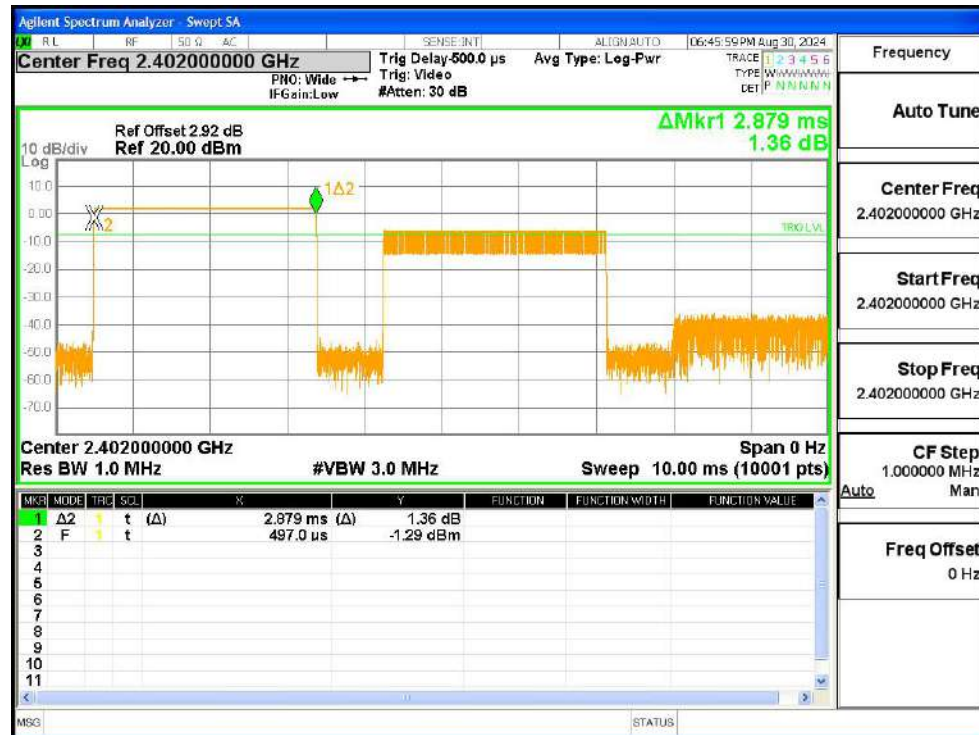
Dwell NVNT 1-DH5 2402MHz Ant1 Accumulated
