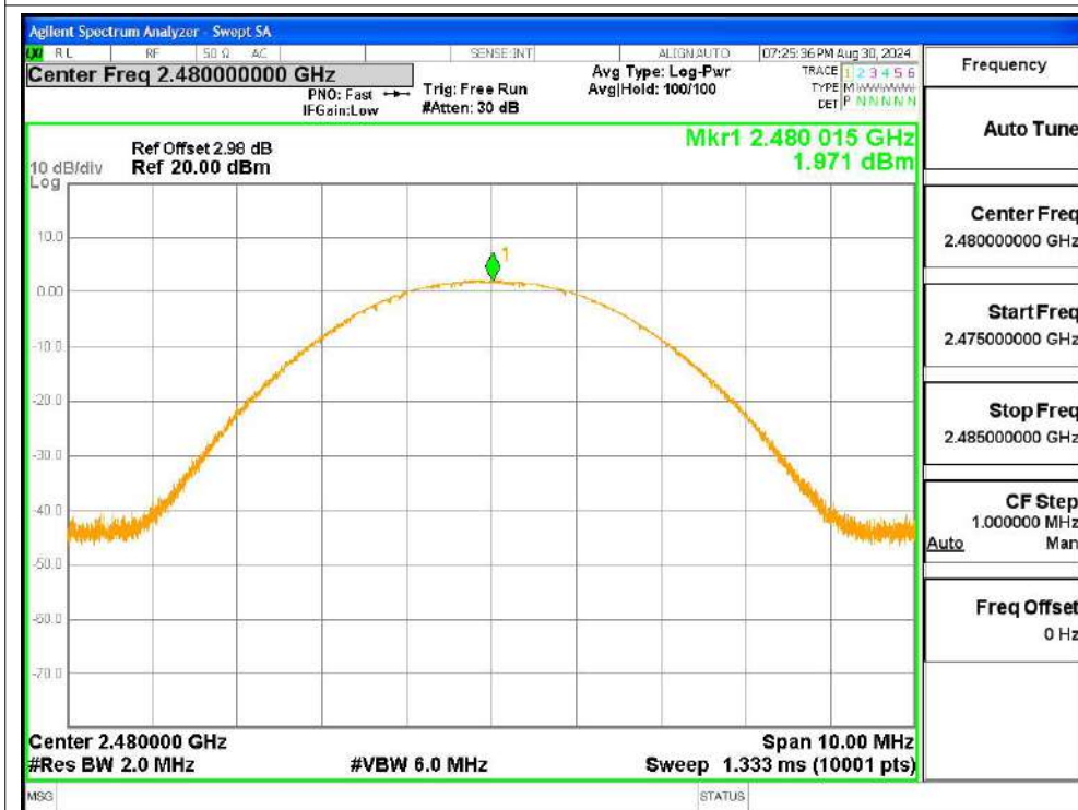
Power NVNT 2-DH5 2480MHz Ant1
