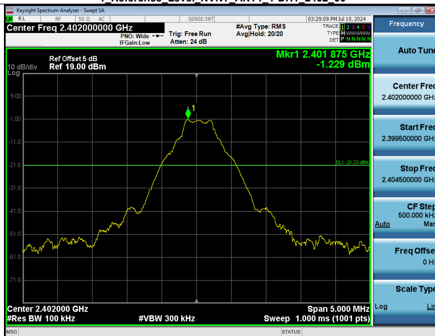
2 Spurious Emissions NVNT ANT1 1-DH1 2402 00
