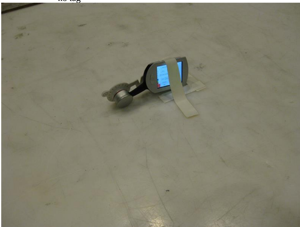
Photo 4.8.2 Test set-up regarding measurement of field strength of fundamental, with tag
