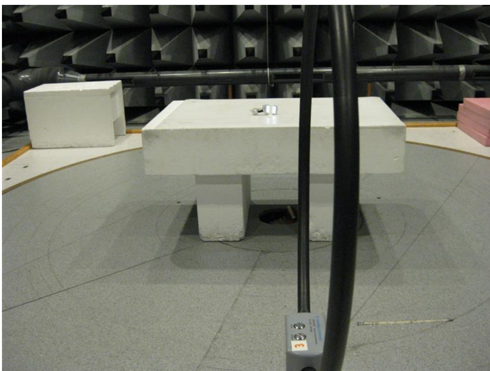
Photo 4.2.2 Test set-up regarding measurement of radiated emission (below 30 MHz).
