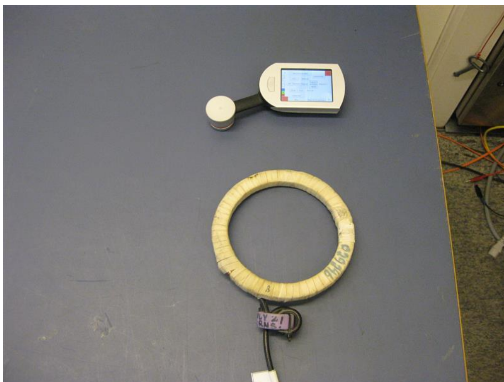
Photo 4.5.2 Test set-up regarding measurement of 20 dB bandwidth
