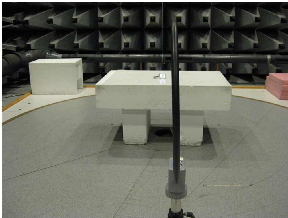
Photo 4.7.3 Test set-up regarding measurement of field strength of fundamental
