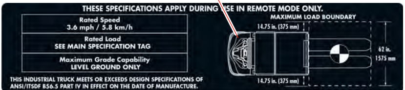
Figure 2: Specification Tag for Model 8510 with Raymond Advance™ Operator Assist Technology
