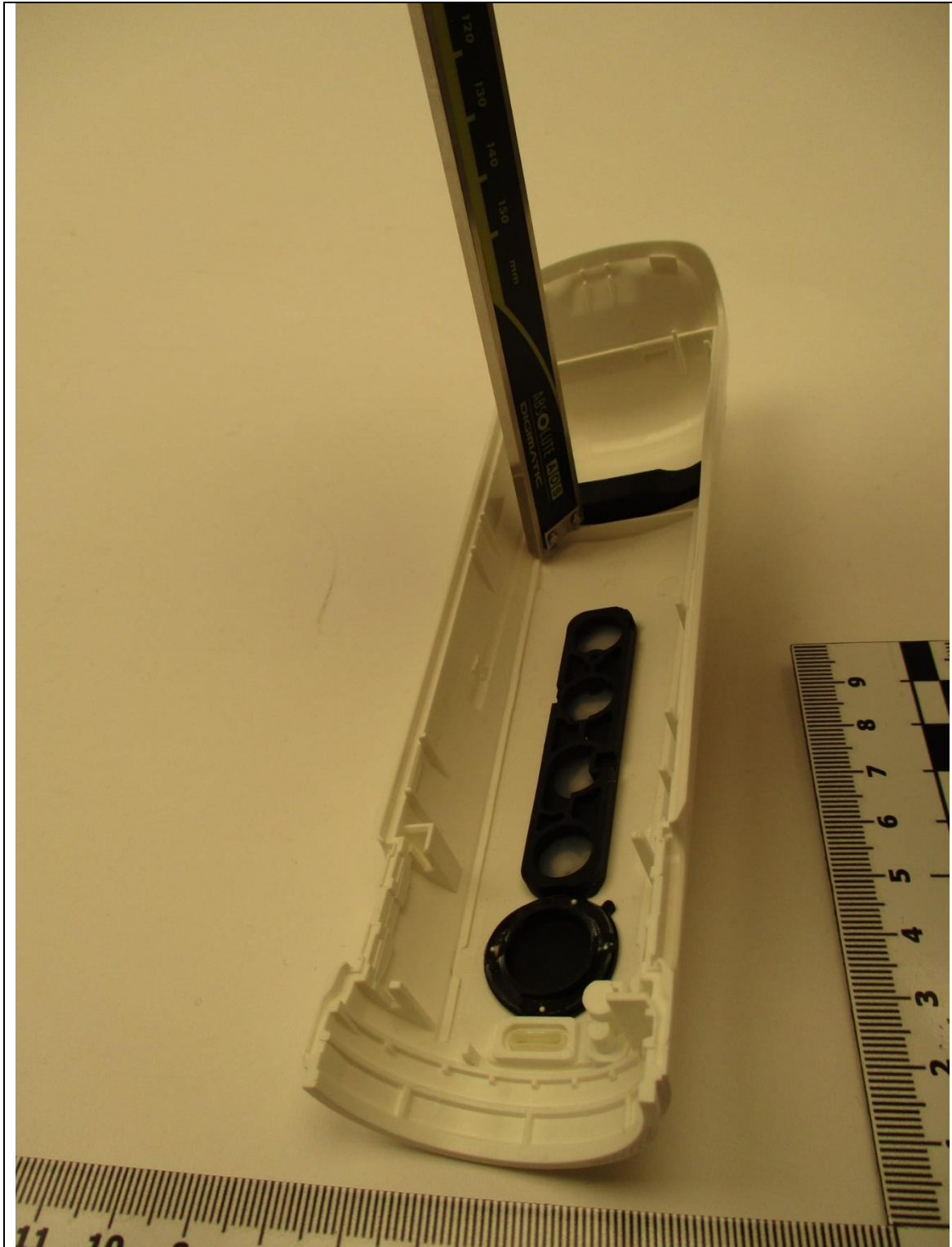
Test setup: Test separation distance measurement ensured by enclosure- BLE
