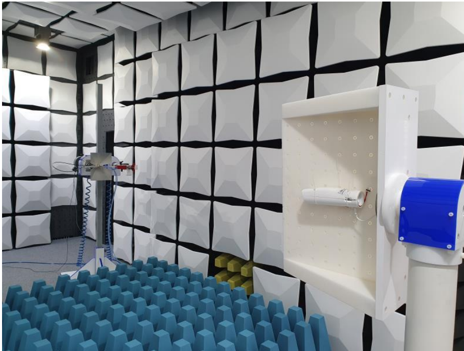
Test Setup: Radiated Measurements (1 GHz to 25 GHz)
