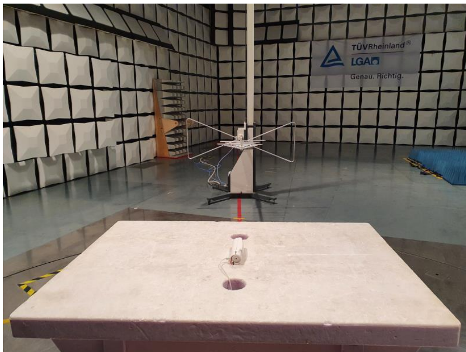
Test Setup: Radiated Measurements (30 MHz - 1 GHz)
