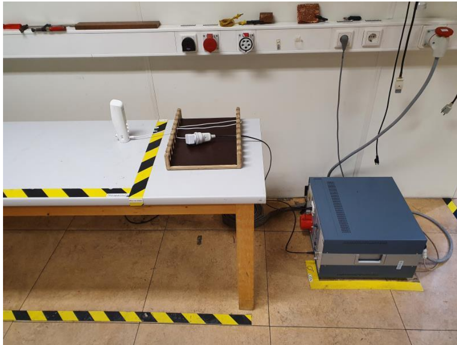
Test Setup: Conducted Emission Measurements
