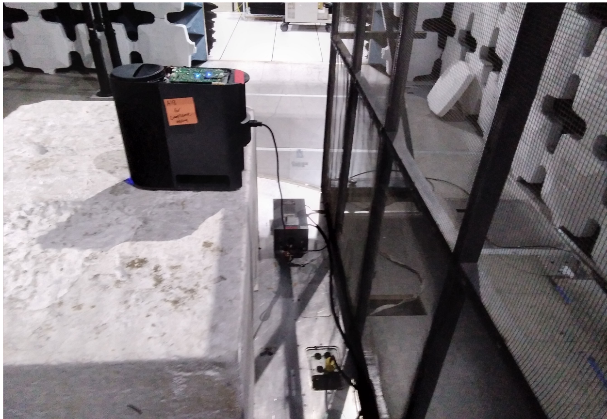
Test Configuration Photograph #2 (Conducted Emissions - Power Port)
