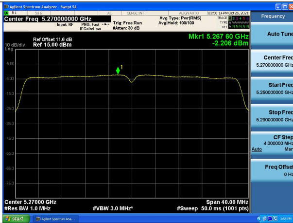
Test Mode:802.11ac VHT40 5270MHz Chain0
