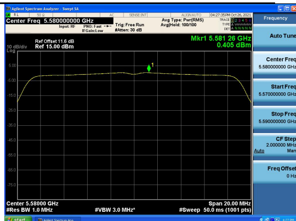
Test Mode:802.11ac VHT20 5580MHz Chain0
