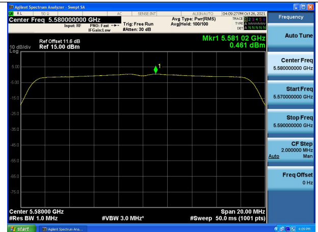
Test Mode:802.11n HT20 5580MHz Chain0
