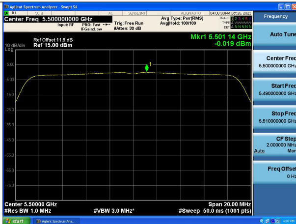
Test Mode:802.11n HT20 5500MHz Chain0
