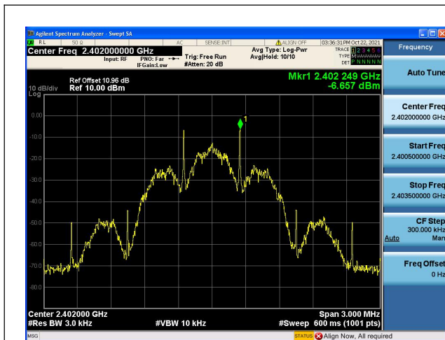
Modulation: Coded 500K 2402MHz
