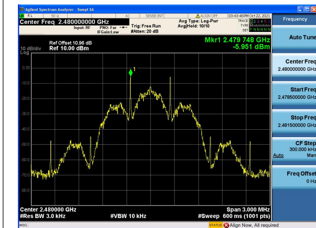
Modulation: Coded 500K 2480MHz
