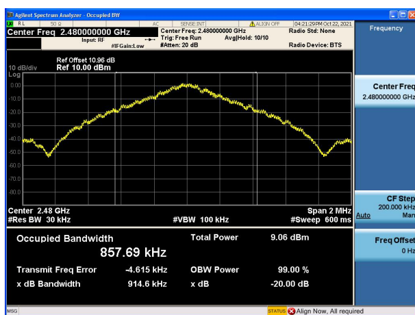
Modulation: GFSK 2480MHz
