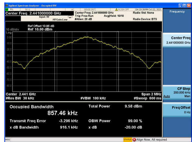
Modulation: GFSK 2441MHz
