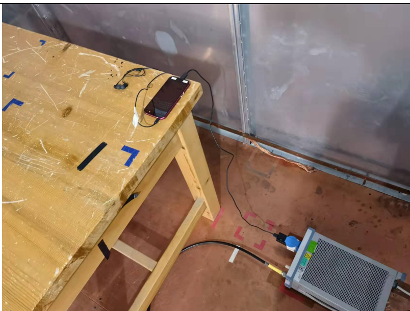
Conducted Emissions Test Setup (with charger)
