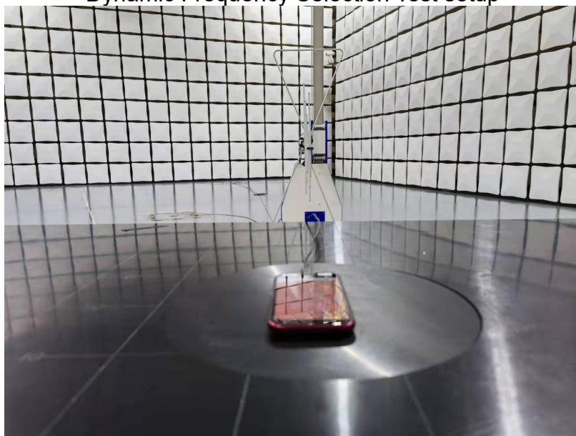
Dynamic Frequency Selection Test setup
