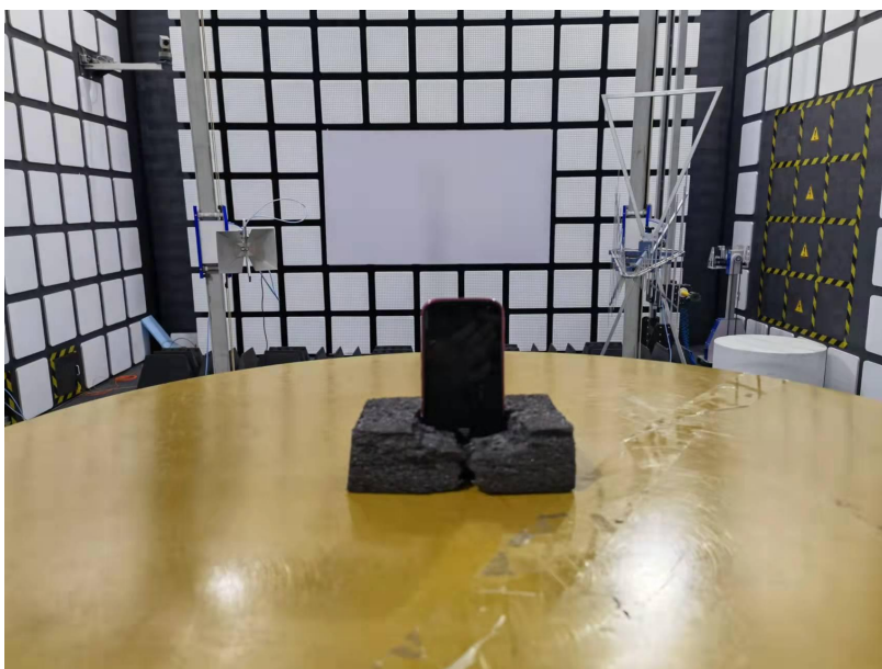
Spurious Radiated Emissions Test setup
