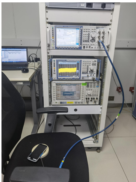
'RF Conducted Test setup (GSM/WCDMA/LTE)
