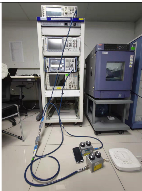
Dynamic Frequency Selection Test setup
