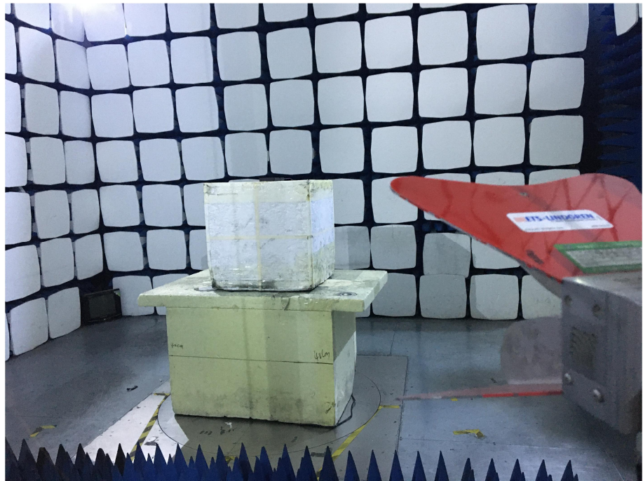
Radiation Emission Test Setup (1GHz to 18GHz)
