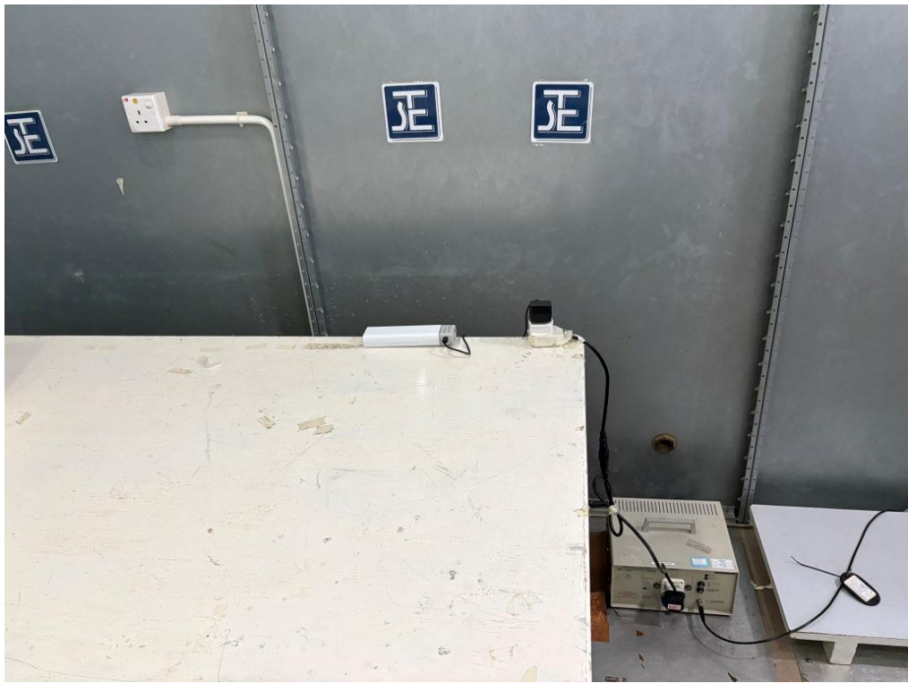
Conducted Emission Test Set Up
