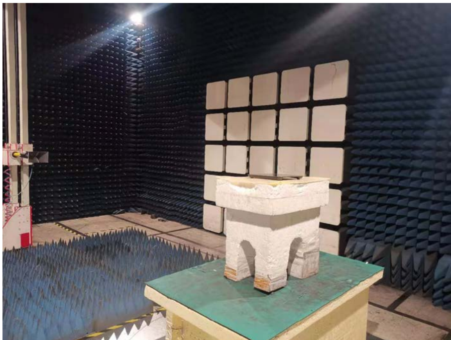
Spurious Emission Test Setup (Above 1GHz)
