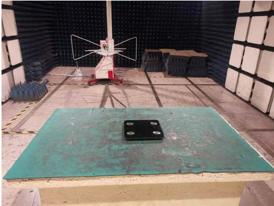
Spurious Emission Test Setup (Above 1GHz)
