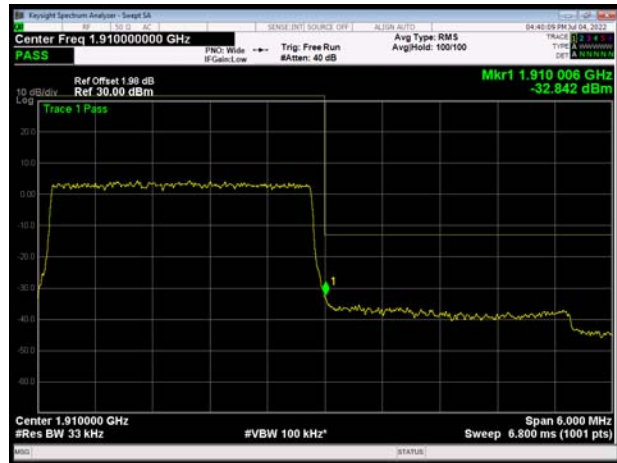
LTE Band 2 5MHz QPSK 1RB CH-High
