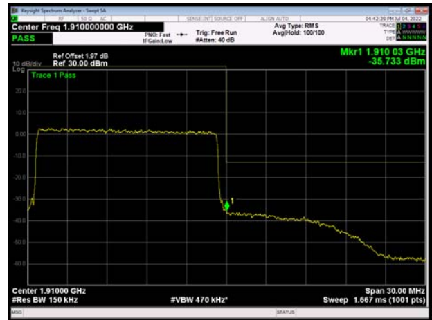
LTE Band 2 20MHz 16QAM 1RB CH-High
