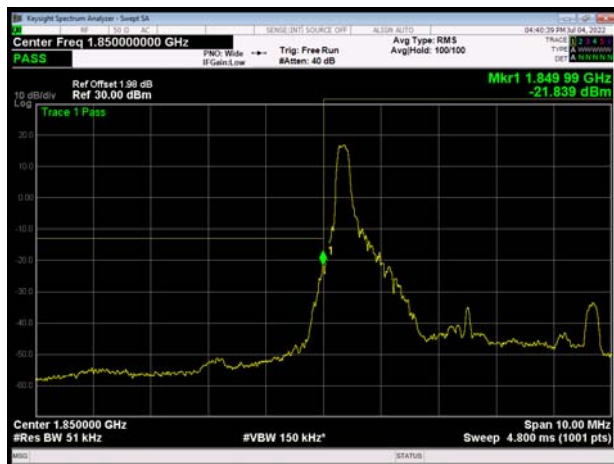
LTE Band 2 5MHz 16QAM 100%RB CH-Low
