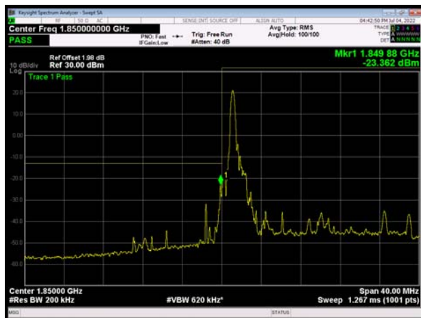
LTE Band 2 20MHz QPSK 100%RB CH-Low
