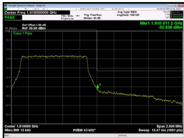
LTE Band 2 3MHz 16QAM 1RB CH-High
