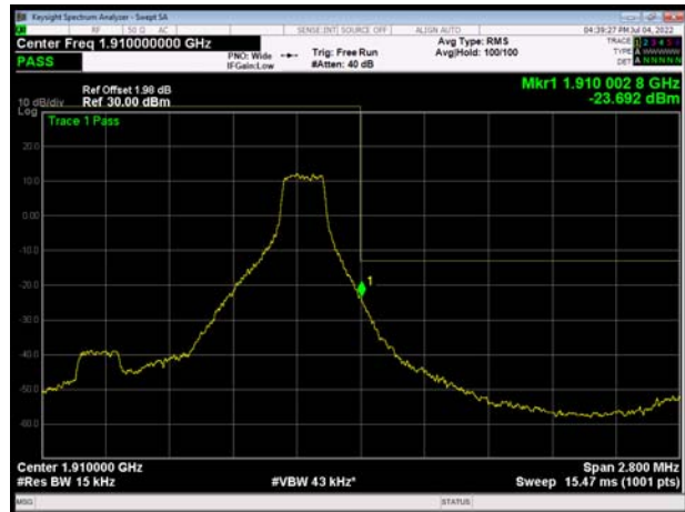
LTE Band 2 1.4MHz 16QAM 100%RB CH-High
