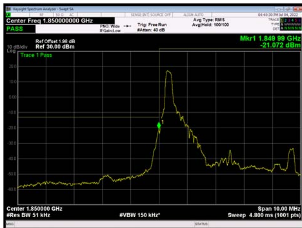
LTE Band 2 5MHz QPSK 100%RB CH-Low
