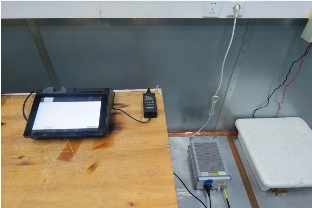
Picture 2 Conducted Emission Test Setup
