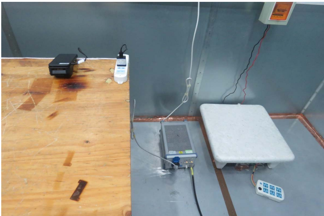
Picture 2 Conducted Emission Test Setup
