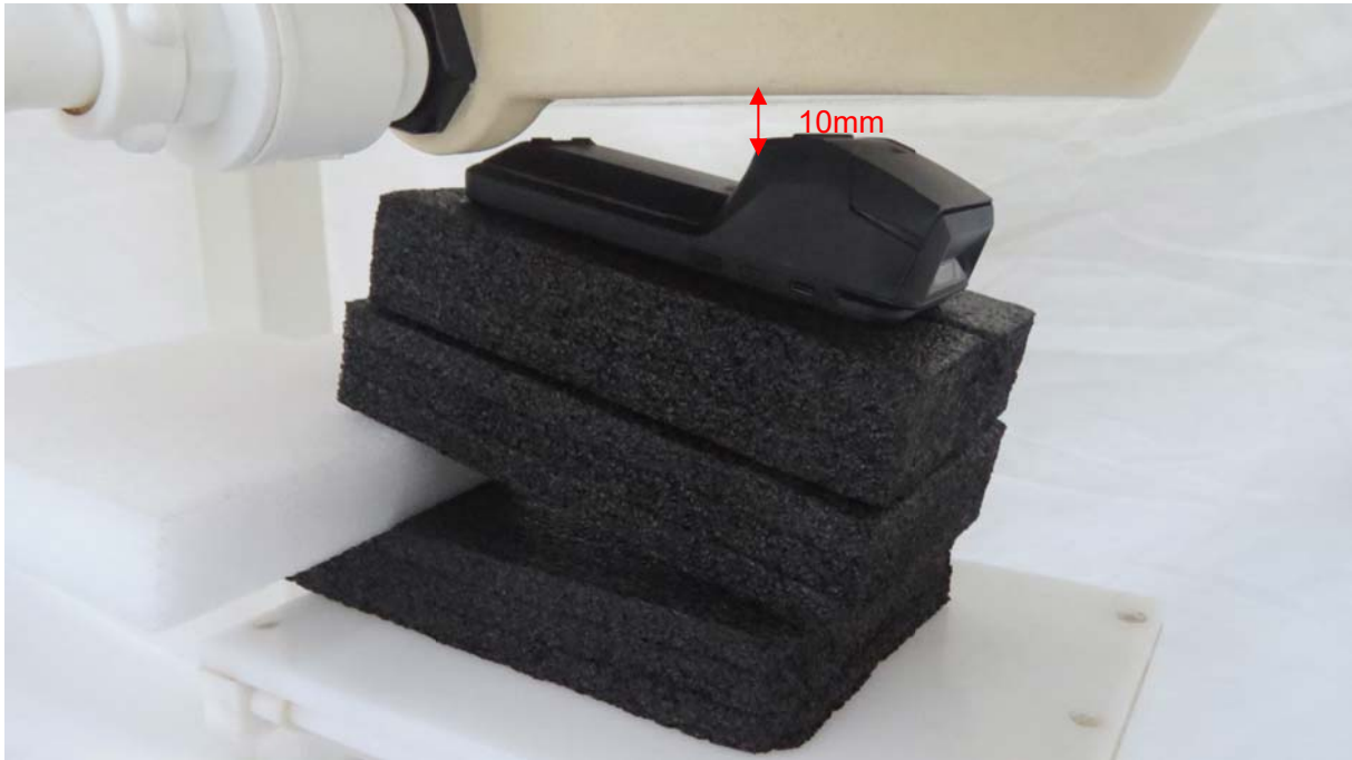
Picture 3: Back Side, the distance from handset to the bottom of the Phantom is 10mm
