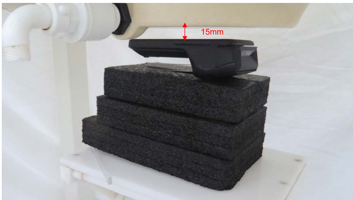
Picture 2: Front Side, the distance from handset to the bottom of the Phantom is 15mm
