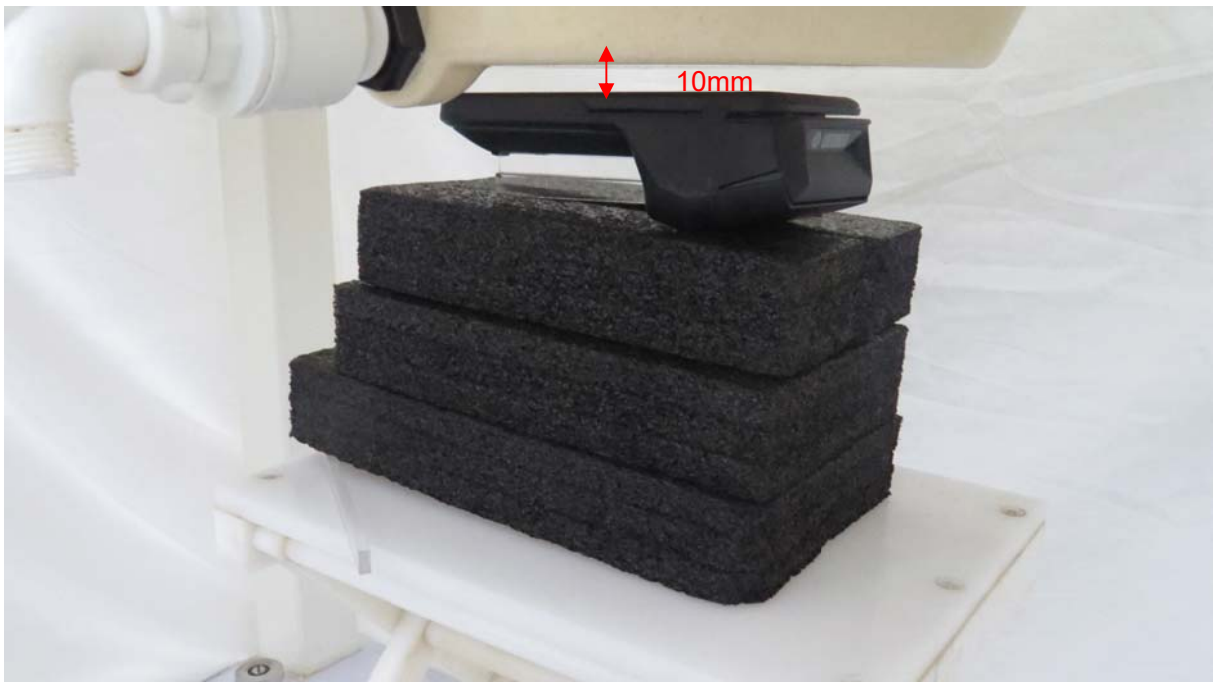
Picture 4: Front Side, the distance from handset to the bottom of the Phantom is 10mm
