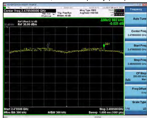
BT 2DH5 CH78, Carrier frequency (MHz): 2480
