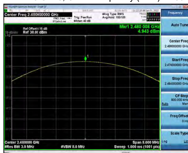
BT DH5 CH78, Carrier frequency (MHz): 2480
