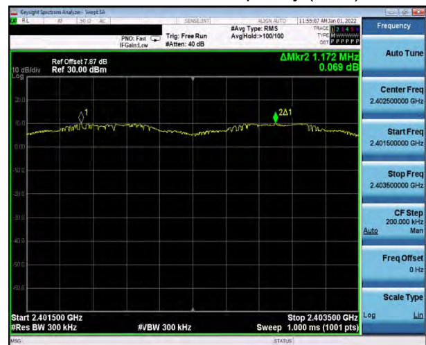
BT 2DH5 CH39, Carrier frequency (MHz): 2441
