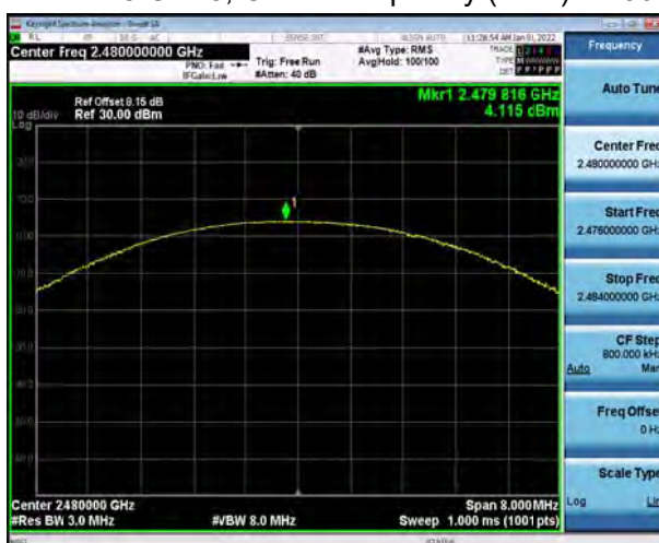
BT 2DH5 CH78, Carrier frequency (MHz): 2480
