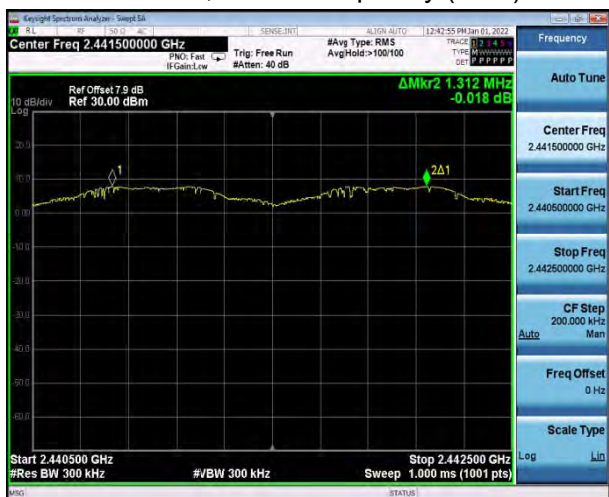
BT 3DH5 CH39, Carrier frequency (MHz): 2441
