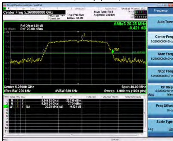
U-NII-2A, 802.11ac VHT20 Carrier frequency (MHz): 5300
