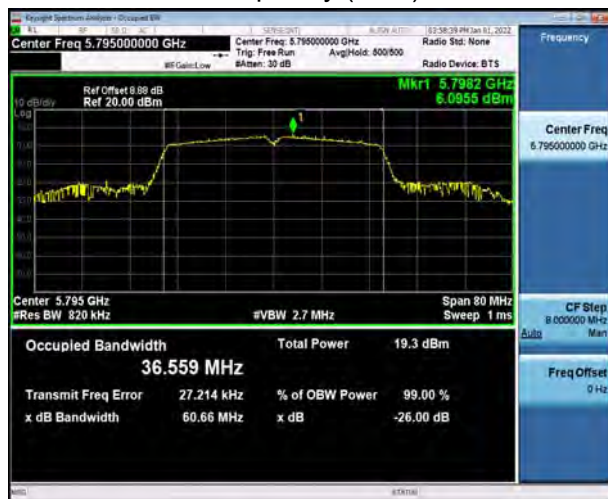
U-NII-3, 802.11ac VHT40 Carrier frequency (MHz): 5755
