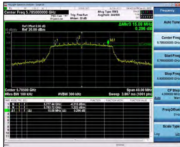
U-NII-3, 802.11ac VHT20 Carrier frequency (MHz): 5825
