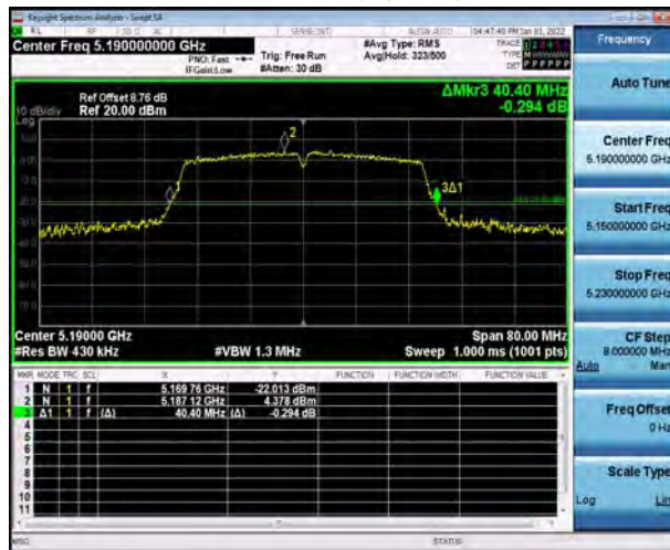
U-NII-1, 802.11ac VHT40 Carrier frequency (MHz): 5190
