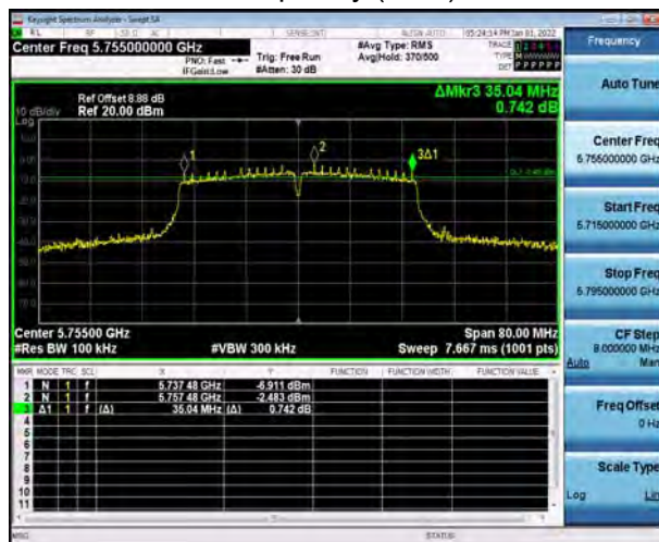
U-NII-3, 802.11ac VHT40 Carrier frequency (MHz): 5755
