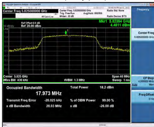
U-NII-3, 802.11ac VHT20 Carrier frequency (MHz): 5825
