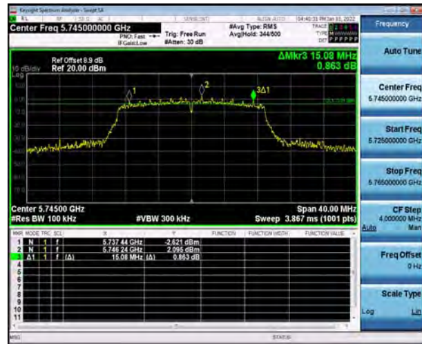
U-NII-3, 802.11ac VHT20 Carrier frequency (MHz): 5785
