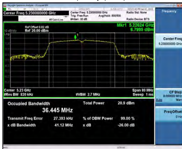
U-NII-1, 802.11ac VHT40 Carrier frequency (MHz): 5190
