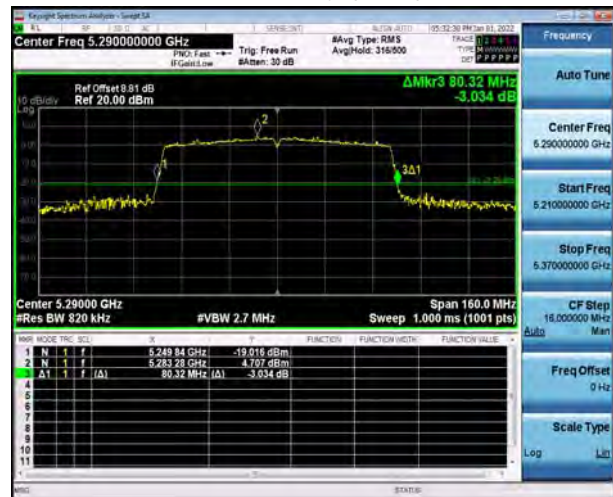
U-NII-2A, 802.11ac VHT80 Carrier frequency (MHz): 5290
