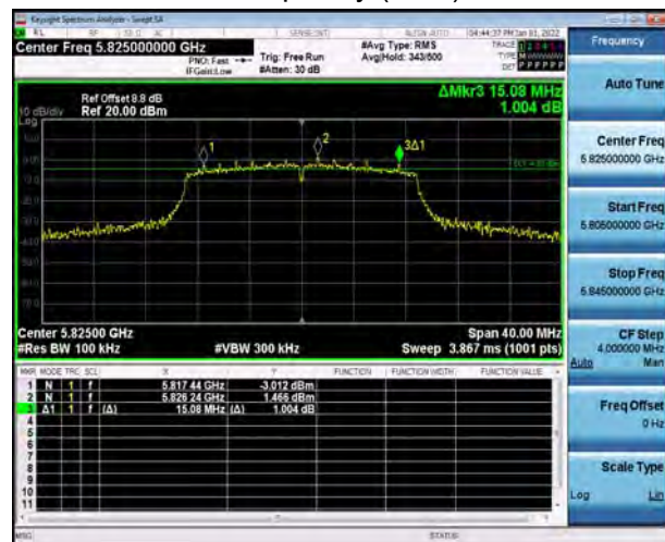
U-NII-3, 802.11ac VHT20 Carrier frequency (MHz): 5825
