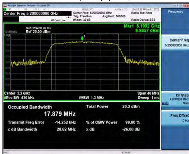
U-NII-1, 802.11ac VHT20 Carrier frequency (MHz): 5240
