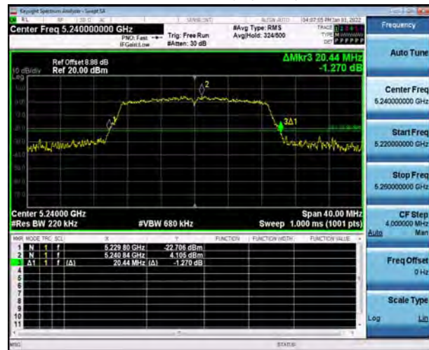
U-NII-1, 802.11ac VHT20 Carrier frequency (MHz): 5240
