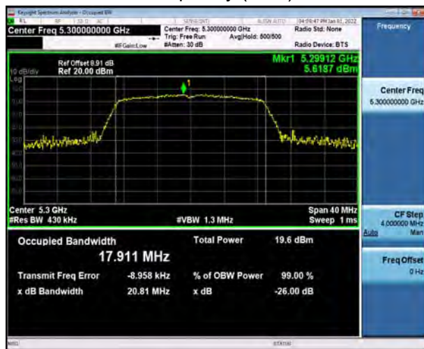
U-NII-2A, 802.11ac VHT20 Carrier frequency (MHz): 5300
