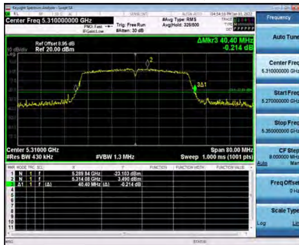
U-NII-2A, 802.11ac VHT40 Carrier frequency (MHz): 5310
