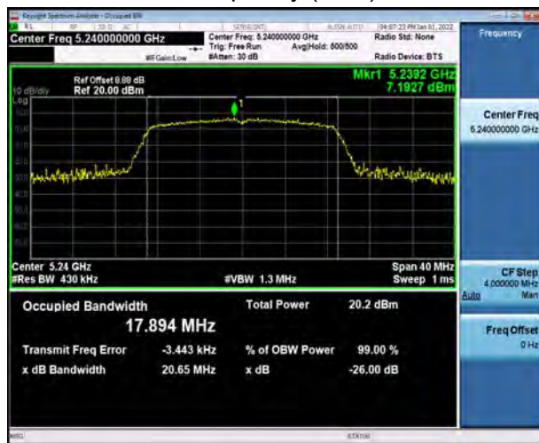
U-NII-1, 802.11ac VHT20 Carrier frequency (MHz): 5240
