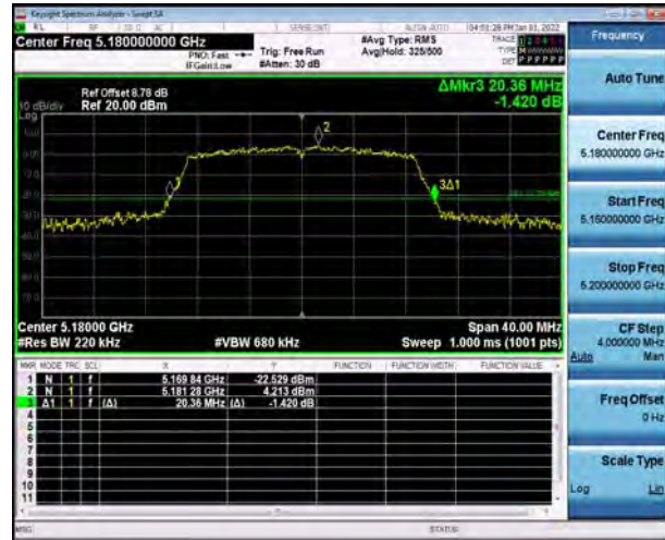
U-NII-1, 802.11ac VHT20 Carrier frequency (MHz): 5200
