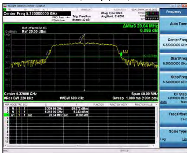
U-NII-2A, 802.11ac VHT20 Carrier frequency (MHz):5260
