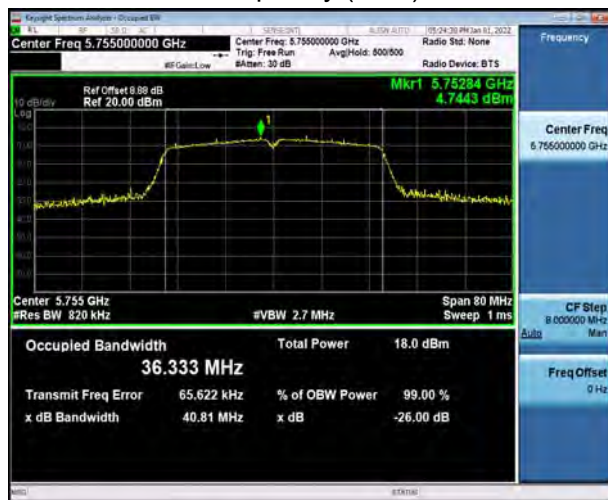
U-NII-3, 802.11ac VHT40 Carrier frequency (MHz): 5755
