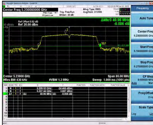
U-NII-1, 802.11ac VHT40 Carrier frequency (MHz): 5190
