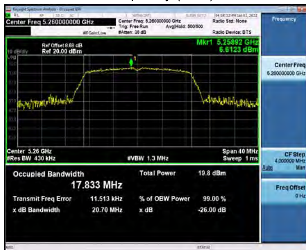
U-NII-2A, 802.11ac VHT20 Carrier frequency (MHz): 5300
