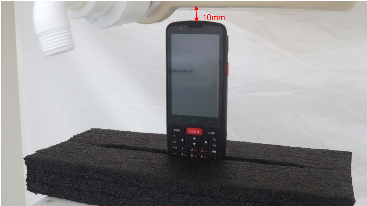
Picture 9: Top Edge, the distance from handset to the bottom of the Phantom is 10mm
