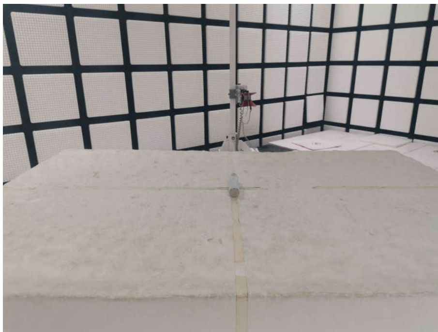
Radiated spurious emission Test Setup-2(Above 1GHz)
