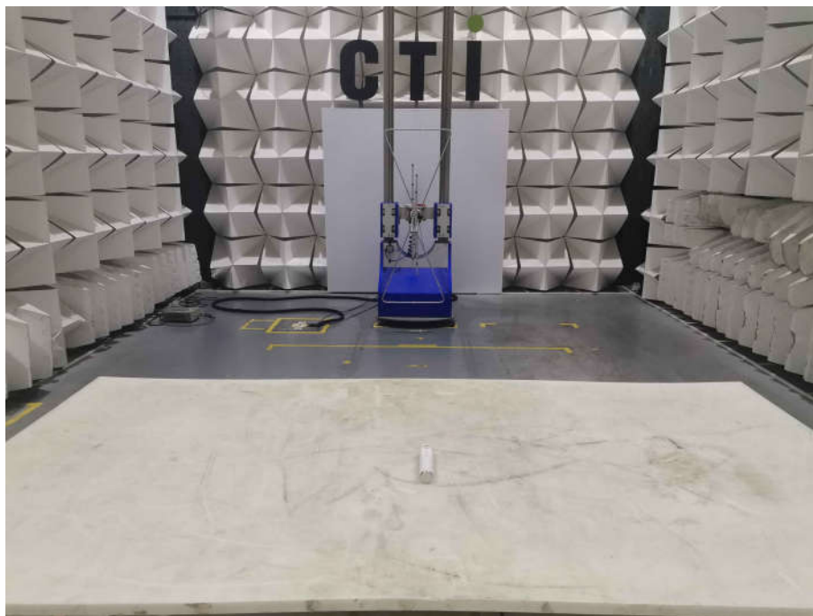
Radiated spurious emission Test Setup-1(Below 1GHz)
