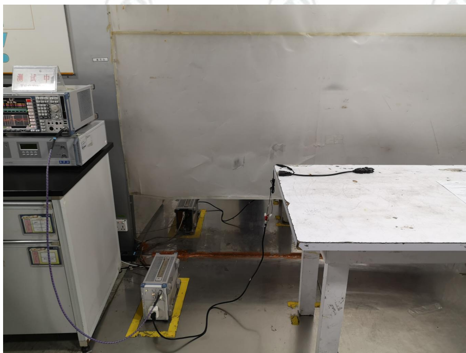
Conducted Emissions Test Setup
