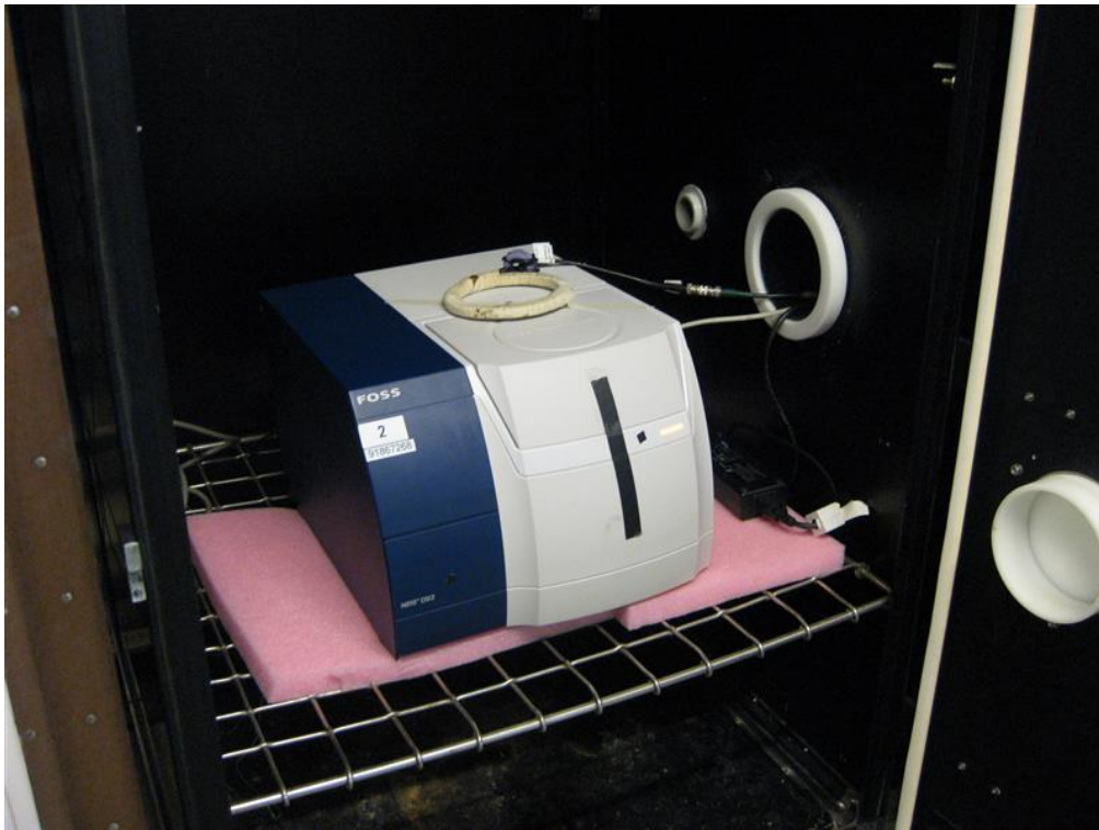
Photo 4.8.1 Test setup regarding measurement of Frequency stability.
