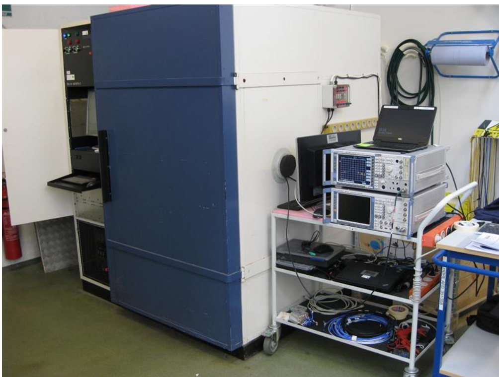
Photo 4.8.2 Test setup regarding measurement of Frequency stability.
