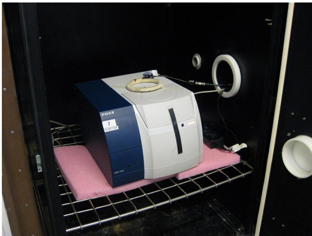
Photo 4.8.1 Test setup regarding measurement of Frequency stability.
