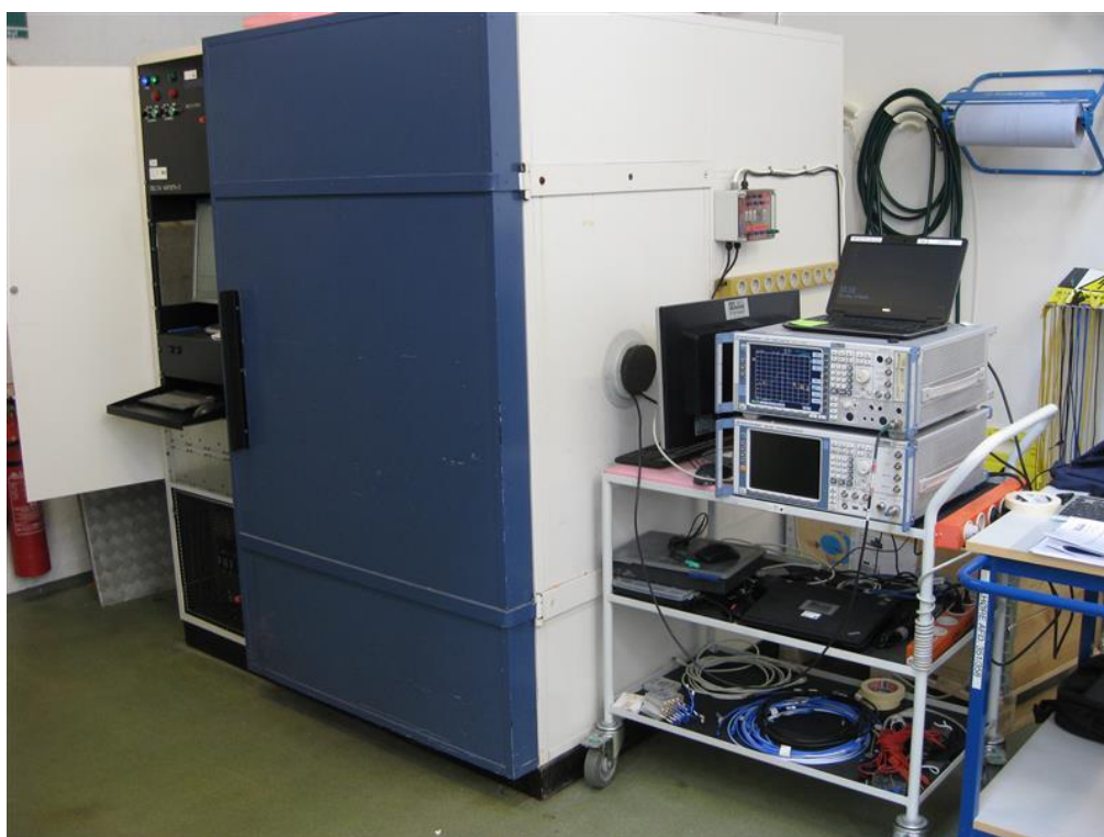
Photo 4.8.2 Test setup regarding measurement of Frequency stability.
