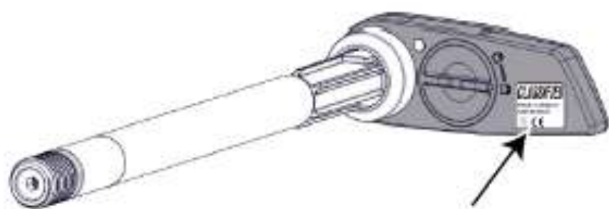
Fig. 2: Smart thru axle label - ITS
