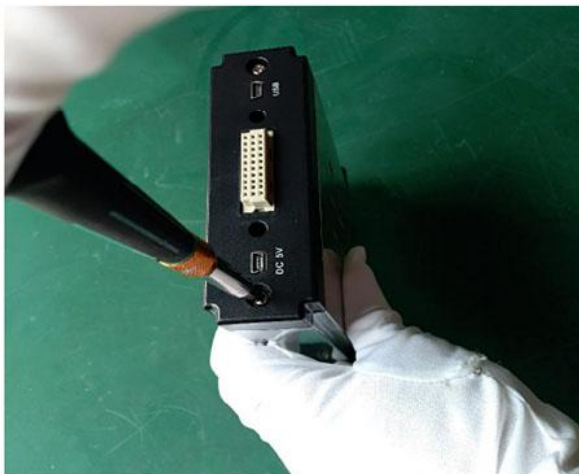
3、 As shown in the figure, unscrew the two fixing screws with a screwdriver to disassemble the entire hard disk box.
