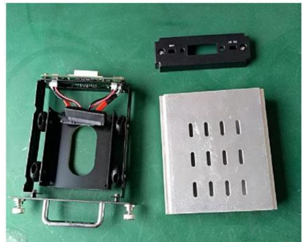
4、 The above picture shows the status of the hard disk box after disassembly.
