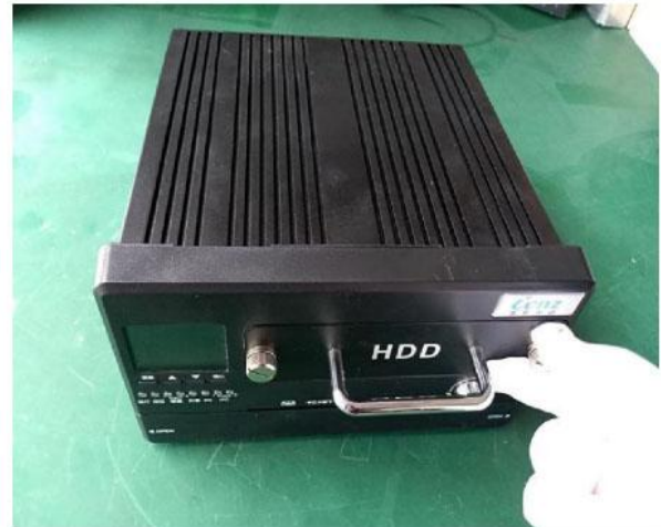
2、 As shown in the figure, open the hard disk lock with the key, unscrew the fixing screw of the hard disk box, and pull out the hard disk.
