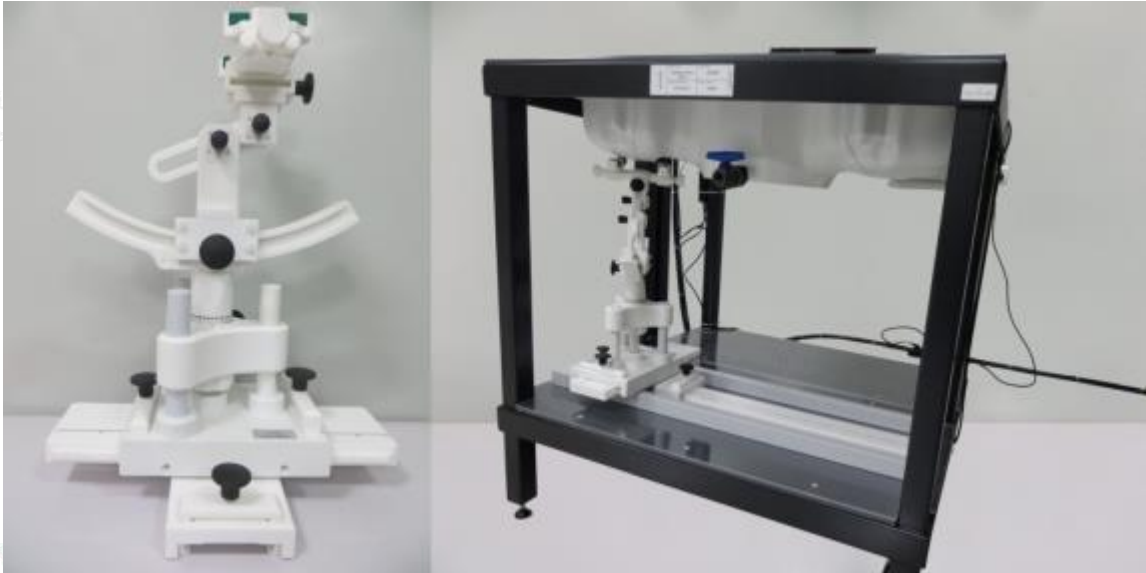
Device holder supplied by SATIMO
