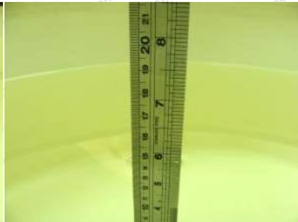
Photo of Liquid Height for Body SAR
