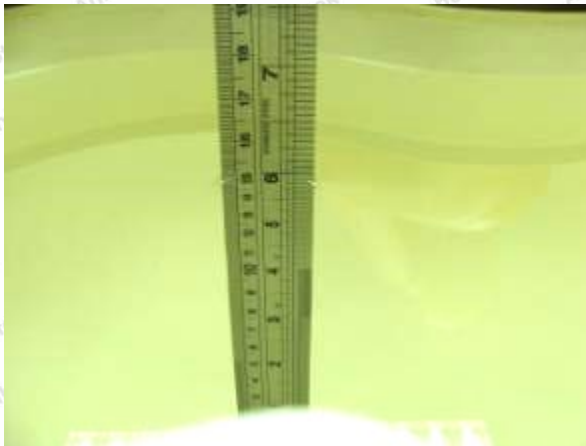
Photo of Liquid Height for Head SAR
