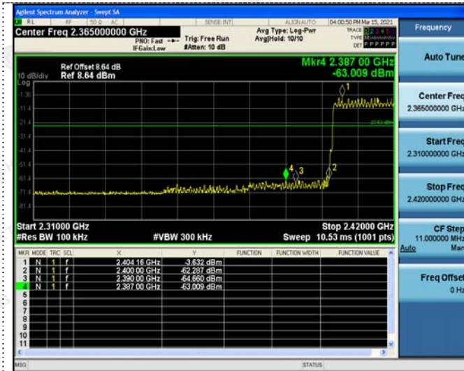
Left Band edge hopping on
