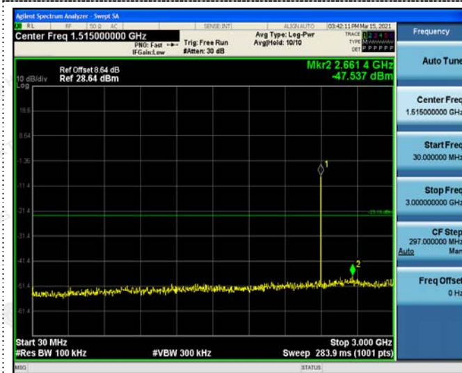
Left Band edge hopping on
