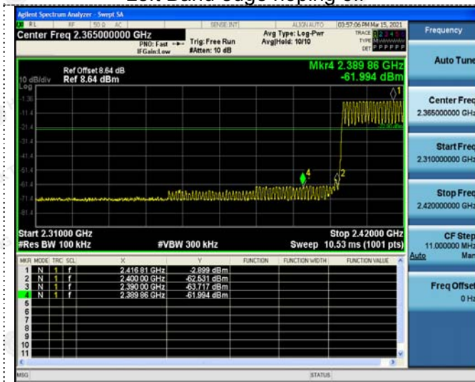
Left Band edge hopping on
