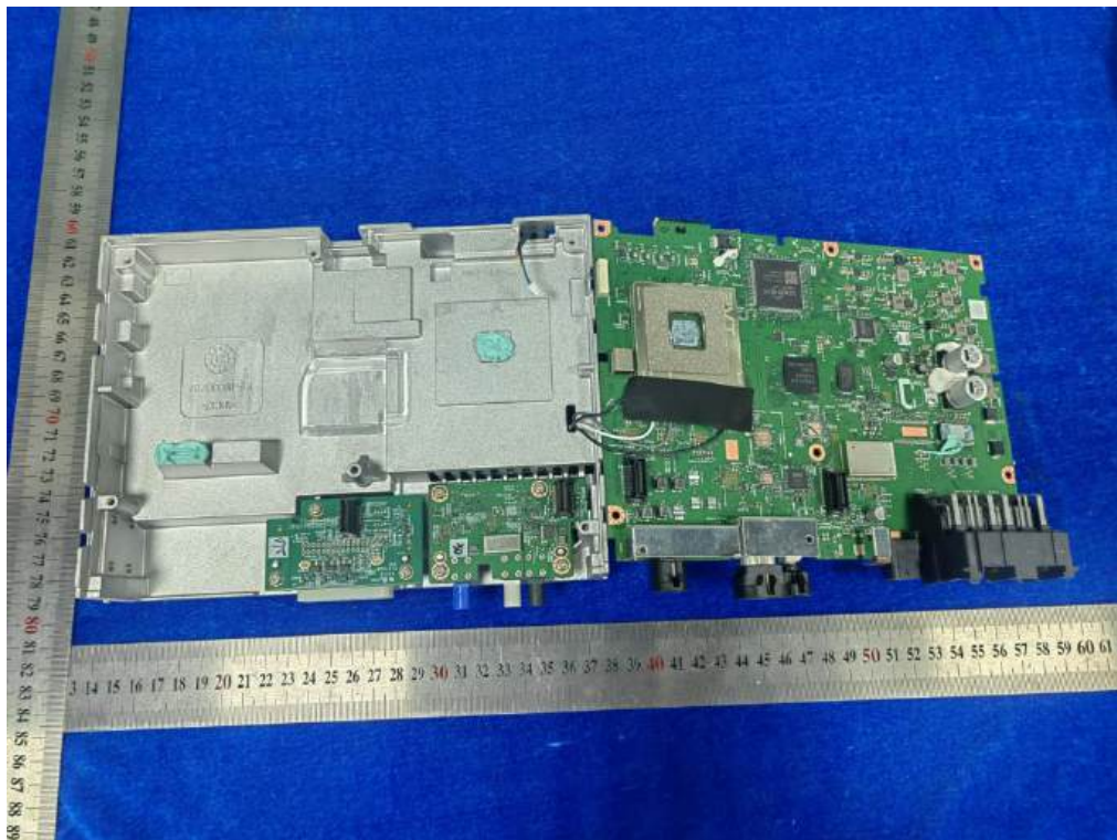
Photo 2: Internal View for PCB
