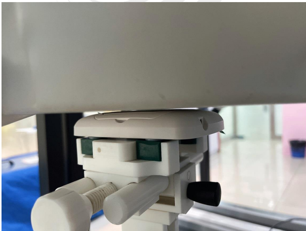
Body Back side(separation distance is 0mm)
