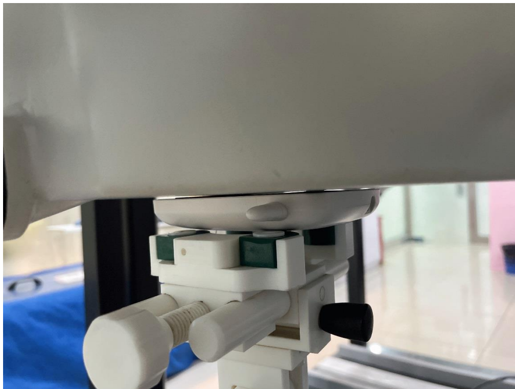
Body Front side(separation distance is 0mm)
