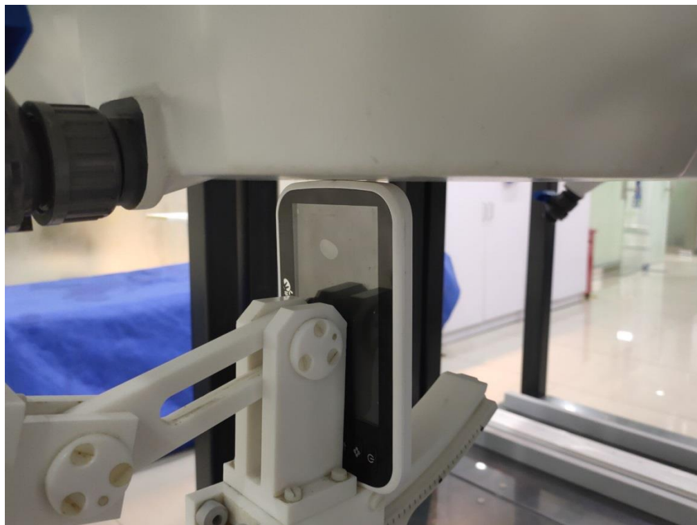
Body Left Side (separation distance is 0mm)
