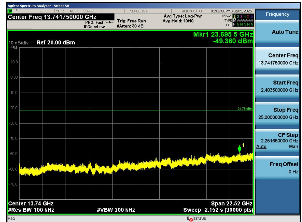
Test_Graph_LE2M_ANT1_2440_2Mbps_Higher Band Emissions
