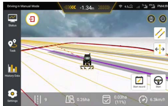
Figure3.5.10 A red dashed line that guides the tractor
