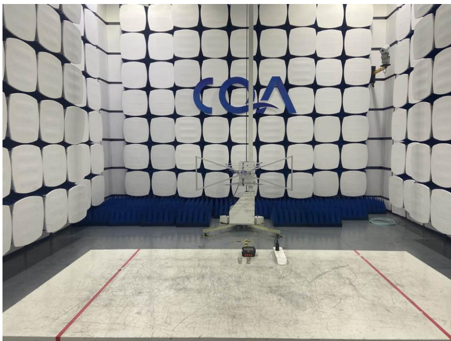
Radiated emission Test Setup (30MHz~1GHz)
